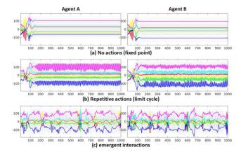
Fig. 2. Three examples of communication patterns between two agents. X and Y axis represent the times steps and joint position values respectively. The colors represent 6 DoFs of the robot used in our study. (a) no actions and (b) repetitive actions between the agents and (c) emergent communicative patterns between the agents
